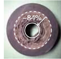
Thick scale piled up in a PVC pipe. (Cross-sectional area decreased 84%)
