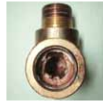
Thick scale piled up in a joint.
